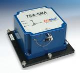
EQMet's TSA-SMA is a very cost-effective 3-channel, 24-bit Strong Motion Accelerograph based on Metrozet's field proven TSA-100S-D24. The three channels of acceleration deliver data at sample rates up to 500sps. With its internal TSA-100S high-performance force balance accelerometers, the TSA-SMA delivers lower-noise performance than competitive units or silicon MEMS-based accelerographs.
